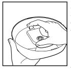
Grip motor with one hand while pressing the locking tab on the motor that holds the lid in place. Remove lid from motor.
