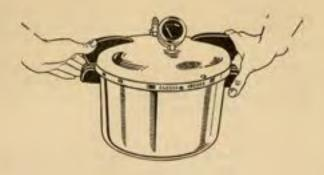
To Close: After placing cover in an open position as designated by the arrow, grasp body and cover handles as per the above diagram, and make a slight turn to the left until handles are parallel and the arrow is opposite the closed position. This will seal your Cooker.
