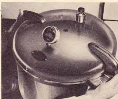
STEP No. 17 —Place cover on Cooker, and lock in closed position. Use maximum heat under it. Be sure petcock valve is wide open.
