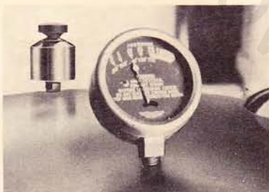
STEP No. 20—Use maximum heat to raise pressure to required point—then lower heat. (On electric stoves, it is necessary to turn heat to "low" just before pressure reaches required point. On coal or wood stoves, Cooker must be moved to cooler place on stove when proper pressure is reached). Start counting processing time the moment required pressure is reached. Pressure should be kept at required point by raising or lowering heat as needed, to eliminate fluctuations in pressure.
